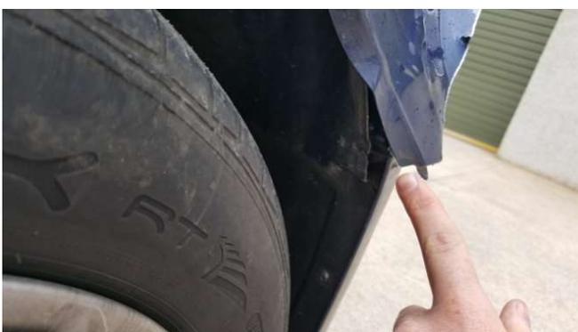
**It is also very helpful to check around other panels that are not immediately obvious such as the wheel arch liner which has been ripped behind the wing, this helps us capture a more accurate assessment and means there are no surprises or delays when further damage is found at a later date**
